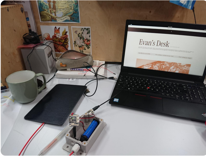
■ The first prototype hosting a simple website over Wifi.
